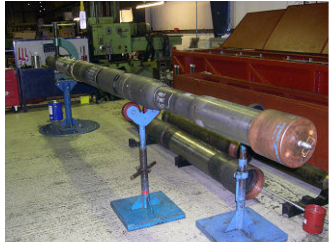
Figure 7: ASV Prepared for Final Test
